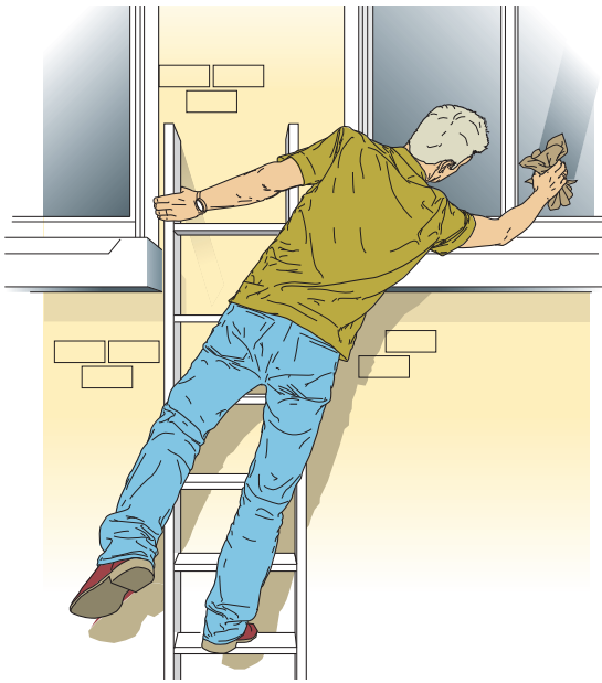
Figure 6 Incorrect - overreaching and failing to maintain three points of contact
